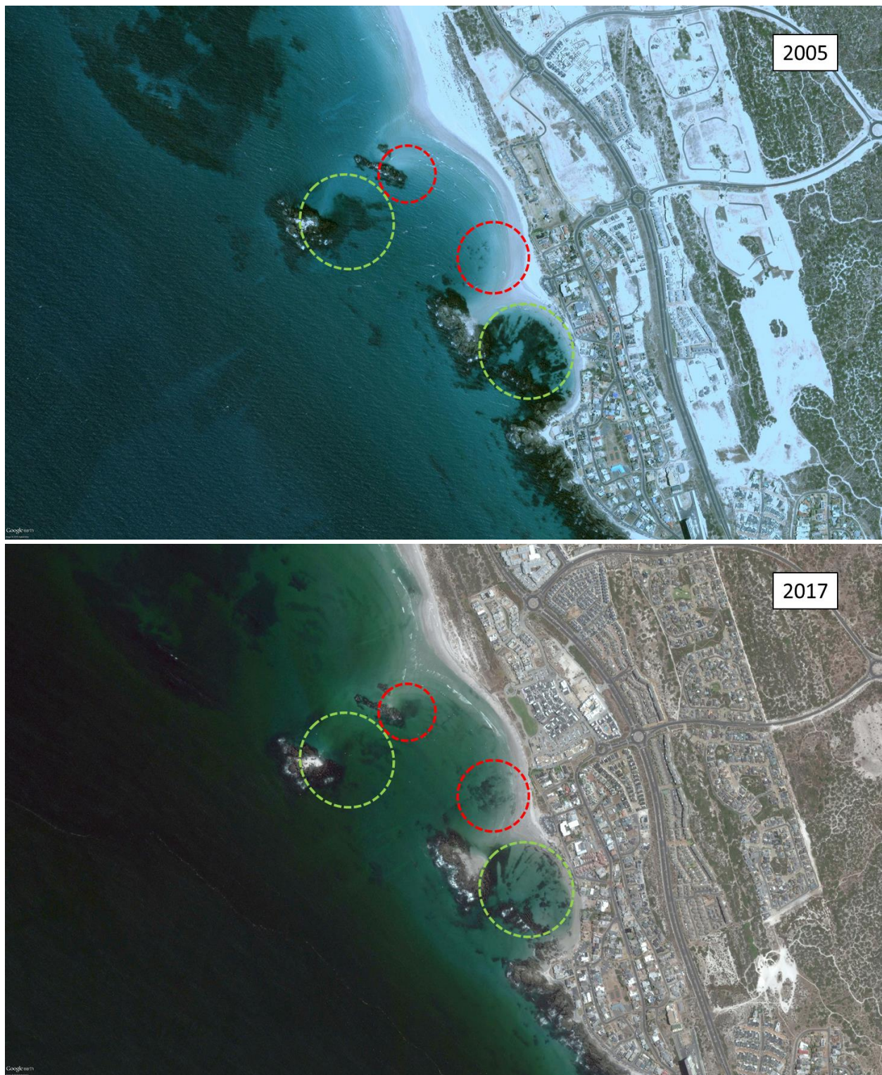
Figure 5-17: Comparison of satellite imagery from 2005 and 2017 showing areas where erosion (red) and accretion (green) have occurred. Erosion/accretion patterns were derived from the extent of sediment cover over rocky outcrops.
